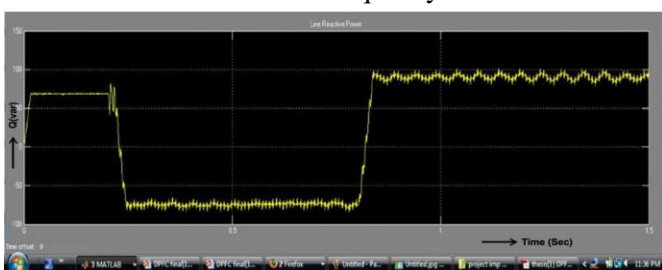
Fig.22: Line reactive power for without DPFC
